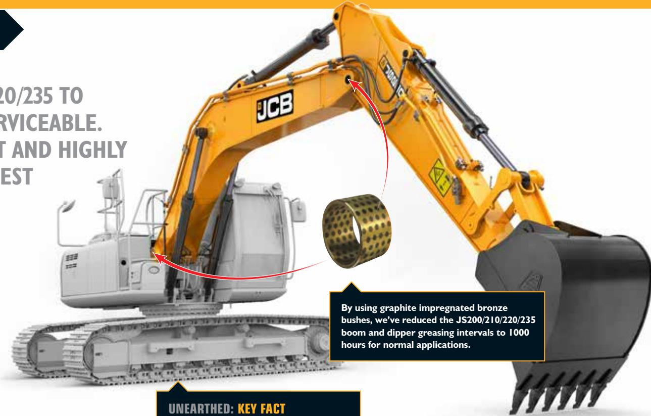
By using graphite impregnated bronze bushes, we've reduced the JS200/210/220/235 boom and dipper greasing intervals to 1000 hours for normal applications.
